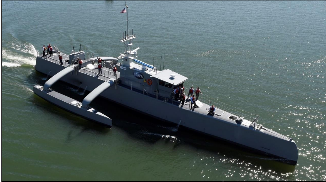
Figure 5. Sea Hunter Prototype Medium Displacement USV
